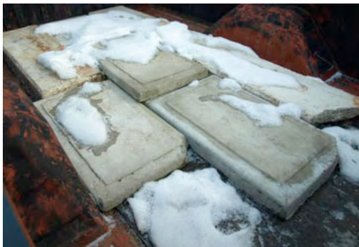
My plan is to put minimal winter miles on the truck – mainly pulling my snowmobile trailer. I'll hose it down regularly to minimize salt damage. The concrete ballast works with the aggressive rear tires and Sure Grip to provide surprisingly good traction on snow.
