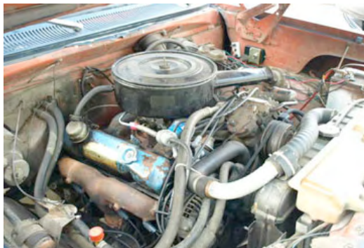
The cast crank 440 is bone stock except for an Edelbrock 750 carburetor residing in place of the original Carter Thermo-Quad.
