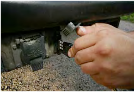
At the vehicle side the harness end from the transmitter is plugged into to the receptacle.
