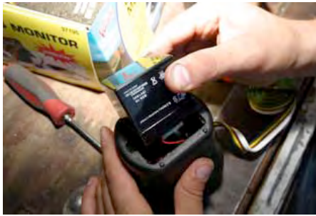
Once the leads are connected, the battery can be installed into the transmitter.
