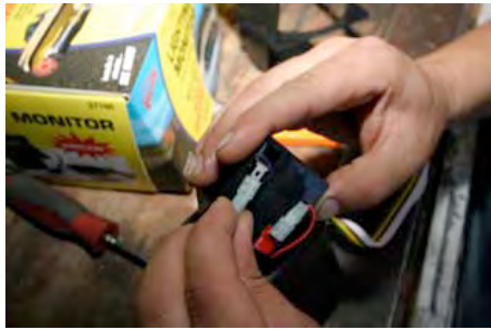
The leads for the battery pack in the transmitter are connected. The leads are easily marked so that you don't cross the polarity.
