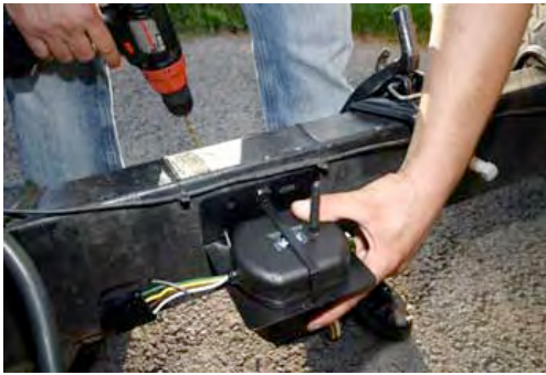
A suitable location is sourced for the transmitter on the frame of the trailer, where it is protected from foreign objects.
