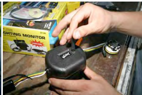
The antenna is then screwed onto the top of the transmitter.
