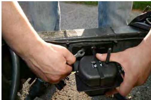
The self-tapping screws are now used to secure the bracket to the trailer.
