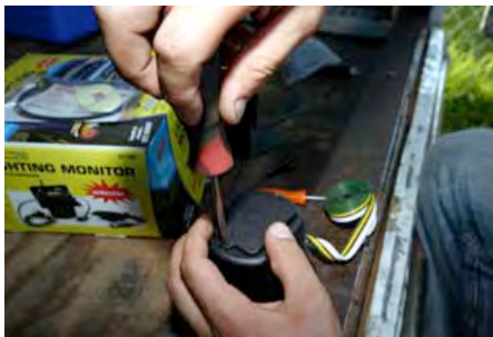
A small Phillips screwdriver is used to perform the final tightening of the cover.
