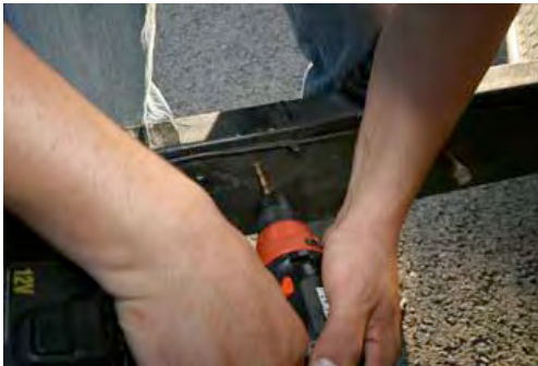
As expected the frame of your trailer is somewhat thick so the drilling may take some patience.
