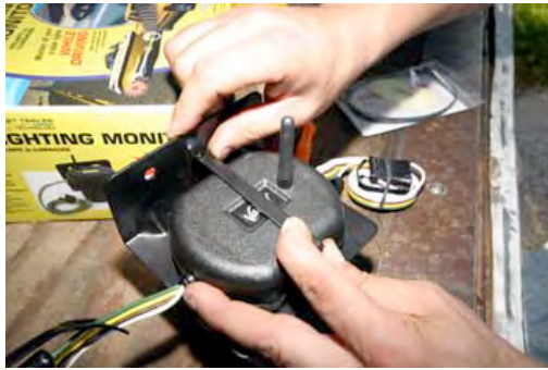
The bar simply press fits into the bracket and secures the transmitter
