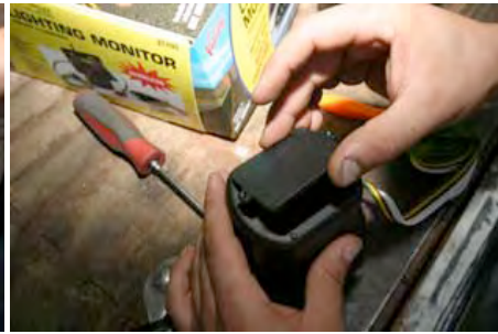
The weatherproof cover is then installed onto the transmitter.
