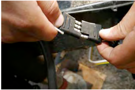
The wire harness plug from the trailer is plugged into the transmitter.
