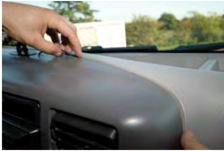
We elected to run the wire down the side of the dash bezel for a clean look.
