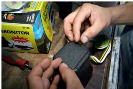
A pair of screws that were supplied with the kit are threaded in, partially by hand at the start.
