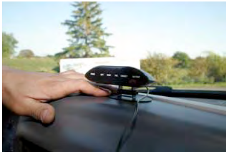
A suitable location for the monitor is sourced on the dashboard of the vehicle.
