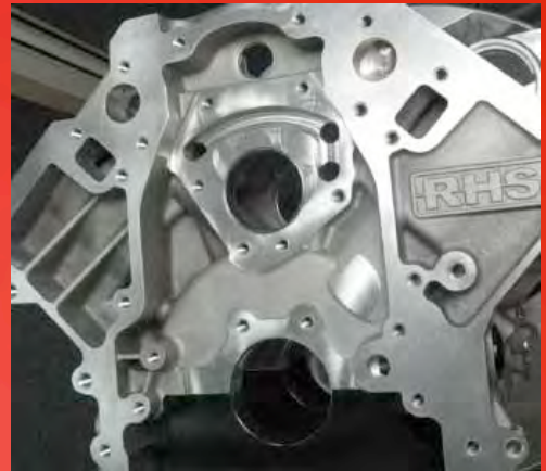
This front view of a production block shows the cam gallery and the timing chain case.
