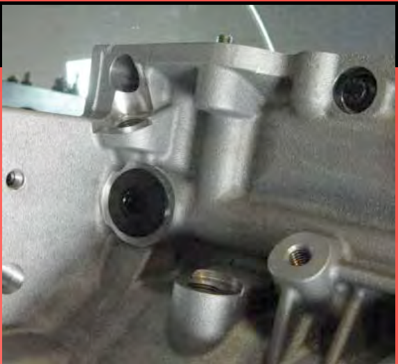
The RHS LS block has an external fixture for the "Knock Sensor" as well as in the stock location.
