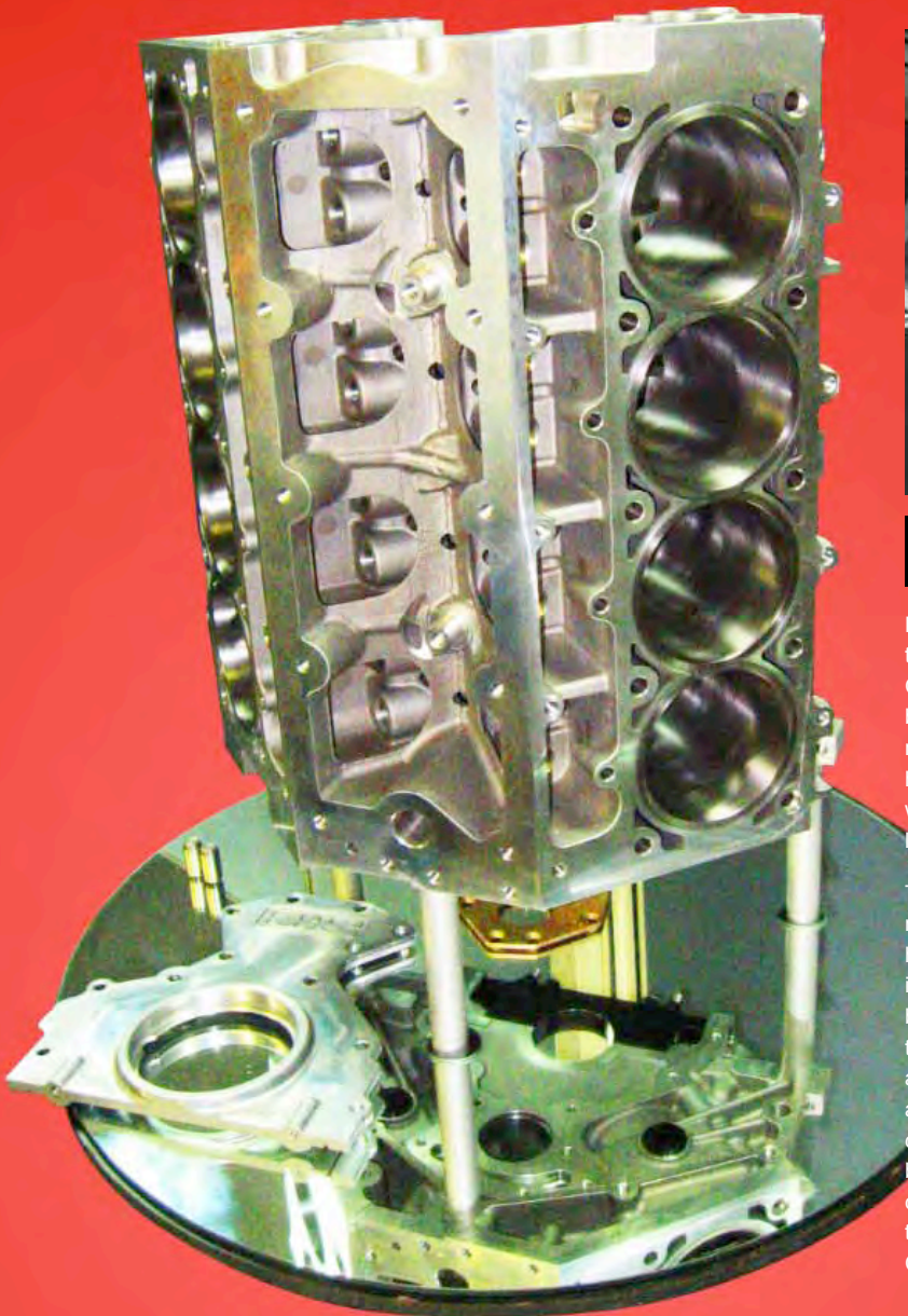
This front view of a production block shows the cam gallery and the timing chain case.
