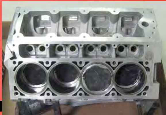
Here is the short block used to build the 700hp dyno test engine. Notice siamesed sleeves.
