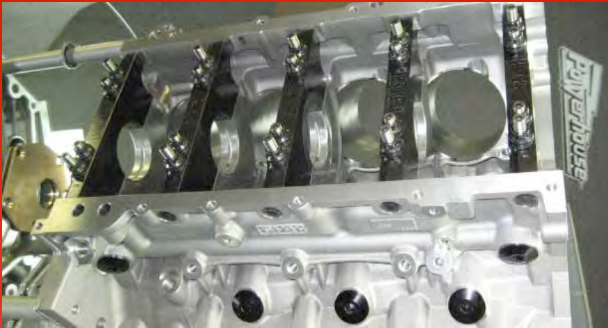
Here is a close-up look at the Crankcase. Notice the six-bolt mains with cross bolting.
