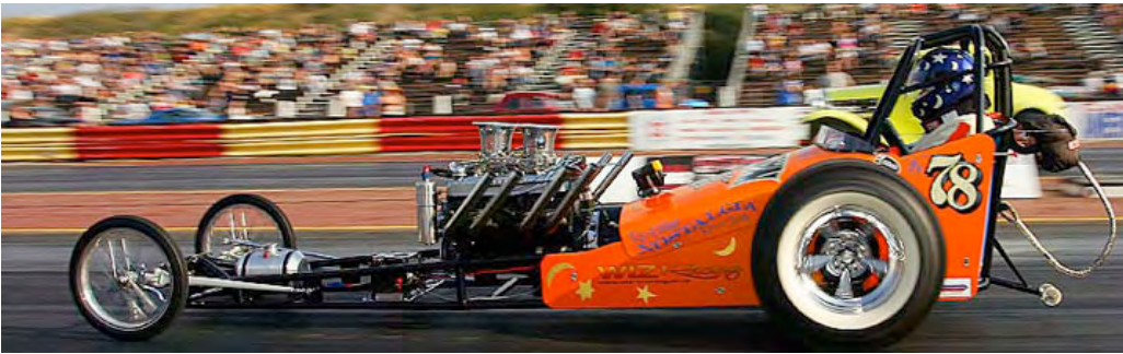
Along with Solley, Keith Crampton is another Wild Bunch Nostalgia Series member with the Wiz Racing 'Soul Town Shaker' slingshot getting the go forward from a 425ci Buick Nailhead.
