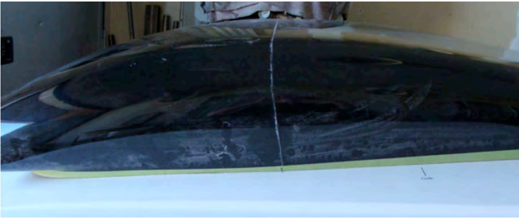
The final fit of the scoop to the hood after contouring.
