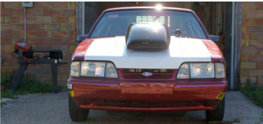
As you can see, the scoop is centered on the hood and will provide quite a bit of room for the carb. The opening is right at the leading edge of the hood.
